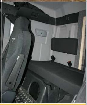
ACTION MOBIL makes it possible to integrate additional seats in the cabin. For this purpose a folding bench ist installed behind the regular seats. Being equipped with headrests and additional seatbelts, the two extra seats are approved by the authorities. The photo shows the extra seats installed in the version "family".
