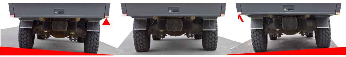
ACTION MOBIL cabins mounted on a chassis with air suspension can now be balanced also in transverse direction
